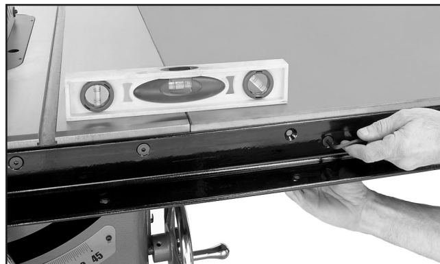
Figure 17. Leveling main extension table.
